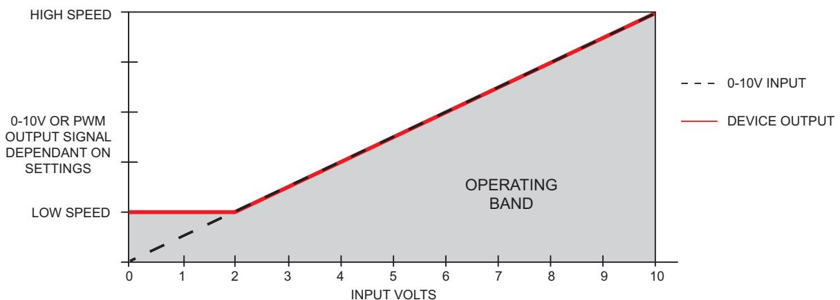
Zero operation set to off, threshold set to 2V.
