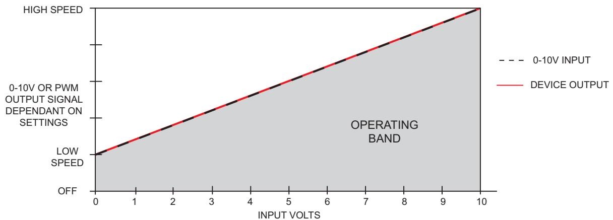
Zero operation set to low speed, threshold set to 2V.
