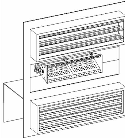
If the pressure drop is too high, in fresh and return air mode, remove or adjust the bypass fresh air and return air damper blank-off panels, which will decrease the pressure drop. If the correct air flow pressure drop is still not achieved adjust the blower drives to decrease the blowers RPM.
