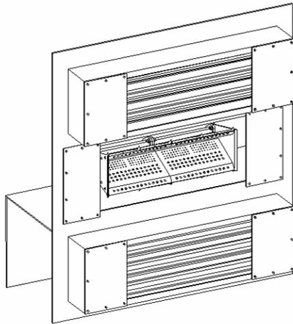
The heater's profile and damper openings are sized to the units designed airflow. While balancing the unit to jobsite static pressures the profile and damper blank-off plates may need to be moved to achieve the correct air flow pressure drop.
