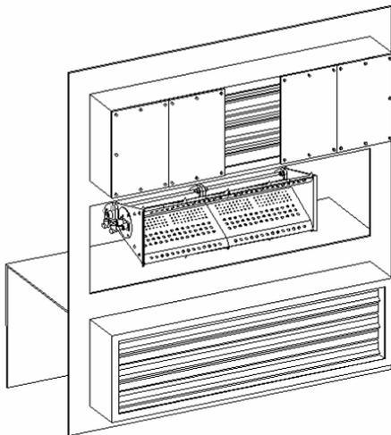
If the pressure drop is too high, in return air mode only, remove or adjust the return air damper and burner profile opening blank-off panels, and add the blank-off panels to the bypass damper, which will decrease the pressure drop.
