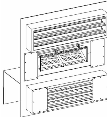
If the pressure drop is too high, in fresh mode only, remove or adjust the bypass damper blank-off panels, which will decrease the pressure drop. The return air damper opening may need to be adjusted to maintain the correct air flow pressure drop when switching back to return air mode.
