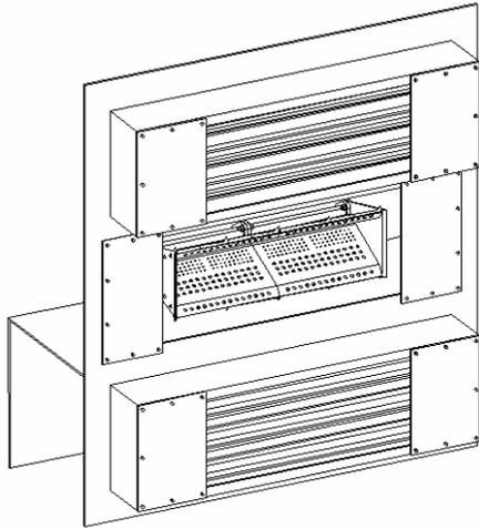
If the pressure drop is too low, in fresh and return air mode, add more blank-off panels to the burner profile opening and bypass fresh air and return air damper, which will increase the pressure drop. (There must be at least 2 inches of area minimum around the burner.) If the correct air flow pressure drop is still not achieved adjust the blower drives to increase the blowers RPM.
